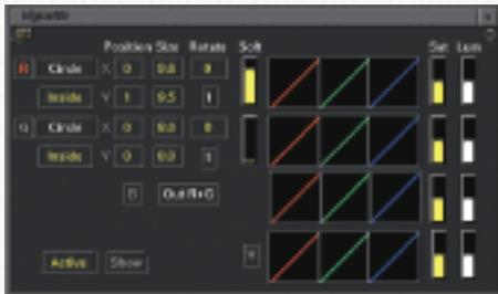
Once "V1" is pressed and the window open, the R and G channels are used to select areas of the picture. There is no colour selection, only the shapes are used; R, G, B and Y are channel names only. The lower orange display (SCC) will show the shape controls, in the same order as for Mega 1. As the R and G channels have their own shape generators, the knobs control whichever of these two channels is currently selected.
